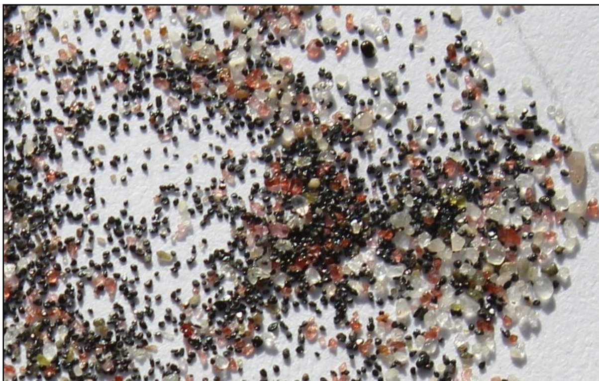
Figure 20: Close-up image indicating the HM and the light minerals. Note the coarse-grained silica grains compared to the finer grained heavy mineral particles. Quartz = large whitish glassy, ilmenite = small black shiny, zircon = very small elongated translucent, garnet = large and small orange-pink-green grains.
