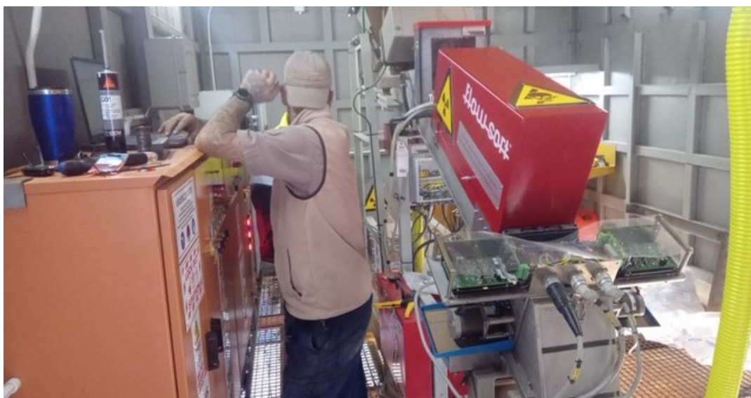
Flowsort X-ray sorting machine processing at the company's concession at Alexkor. Source: Company
